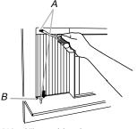
A. #10 x ¾" round-head screw B. Hole for #10 x ¾" round-head screw
